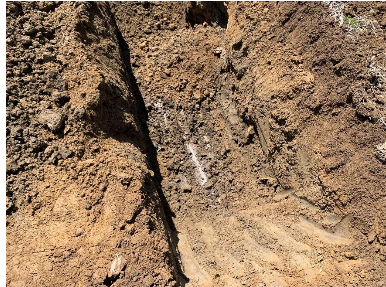
TP-4 on excavation ended on bedrock
